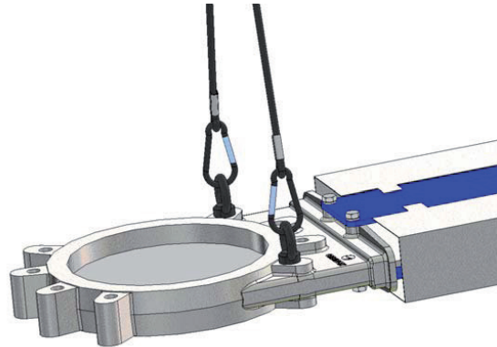
Fig. 1 Suggested Handling with Eyebolts
