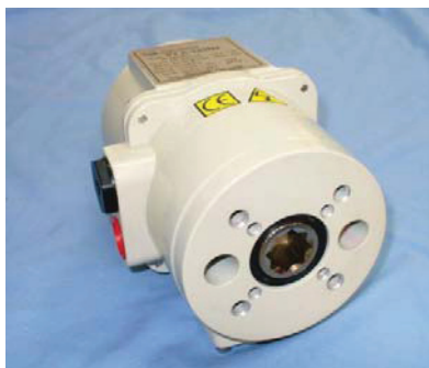
ISO F07 Mounting Detail, 5mm socket override and 8 point 17mm female drive on P0445 Series actuators.
