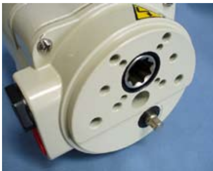
ISO F03/F05 Mounting Detail, 8mm socket override and 8 point 14mm female drive on P1 Series actuators.
