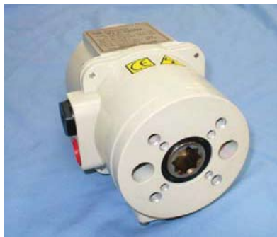
ISO F07 Mounting Detail, 5mm socket override and 8 point 17mm female drive on P1A Series actuators.
